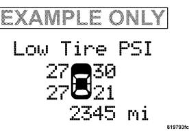
Should this occur, you should stop as soon as possible and inflate all of the tires with low pressure (including those flashing in the EVIC graphic) to the vehicle's recommended cold placard pressure value. Once the system receives the updated tire pressures, the system will automatically update, the graphic display in the EVIC will stop flashing, and the TPM Telltale Light will
